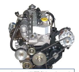
Da-Yeh university advanced vehicle technology research center (AVTRC) is a pioneer in advanced diesel engine development in Taiwan. AVTRC developed a 2.5-liter, direct fuel injection diesel engine to power vehicles, forklifts, and electric generators.
